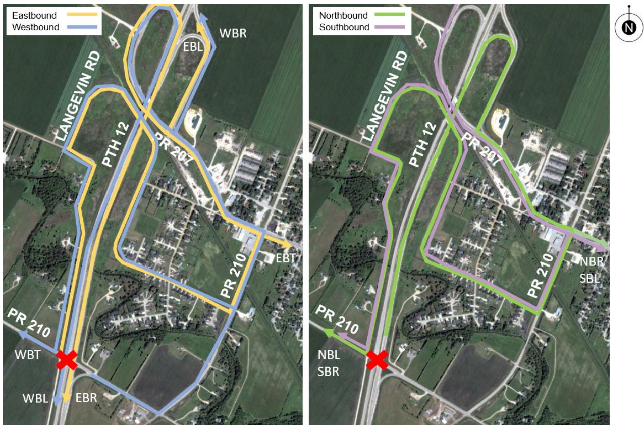
Figure 6.5.1: Re-routing of traffic with intersection full closure
